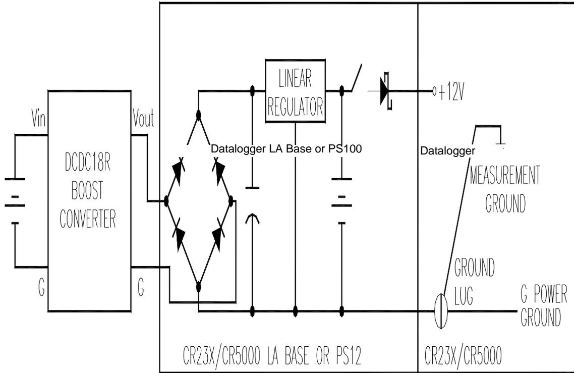
Figure 4. Schematic of Charging and Grounding Circuitry
